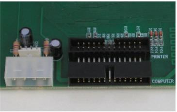
Fig.1.2.1.3: Analyzer Connectors
