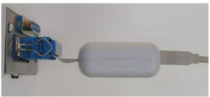
Fig.1.2.5.1: How to connect the USB adapter
