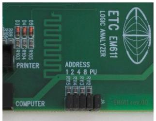
Fig.1.2.1.1: The jumpers layout
