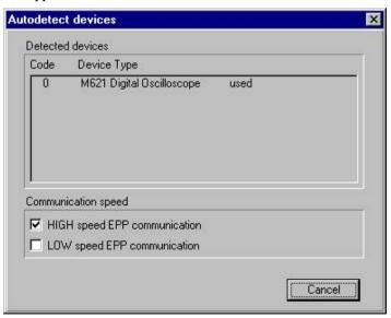
Besides the list of devices, software also displays the EPP communication status in the lower side of the window. Quality of communication depends on several factors, such as cable length, computer features, etc.
