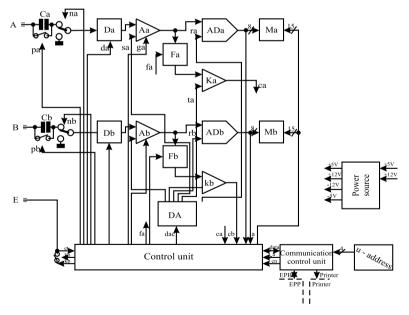
The waveform's digitized pattern is stored into Ma (Mb) memory.
