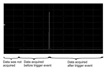
Editable area next to the right of the button allows user to set the number of samples to be collected after trigger event occurs. It also displays the current value. User can change this value by clicking on little arrows right next to the field. Value changes with step of 512. This means that you can divide data from 512 before trigger event and 32000-512=31488 after trigger event to 32000 before trigger event. Place, where trigger event occurs, oscilloscope highlights by vertical red line.
