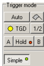
Fig. 4.8.2. – Trigger mode controls with separate hold controls
