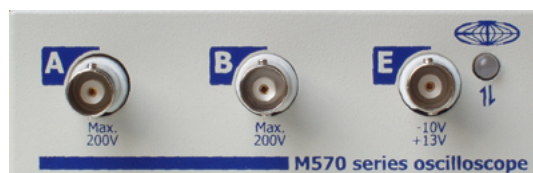
Fig. 3.1.1.1. – Front panel of the M570 series oscilloscope
