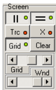
Fig. 4.3.1. – The cursors and grid controls
