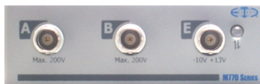
Fig. 3.1.3.1. – Front panel of the M770 series oscilloscope
